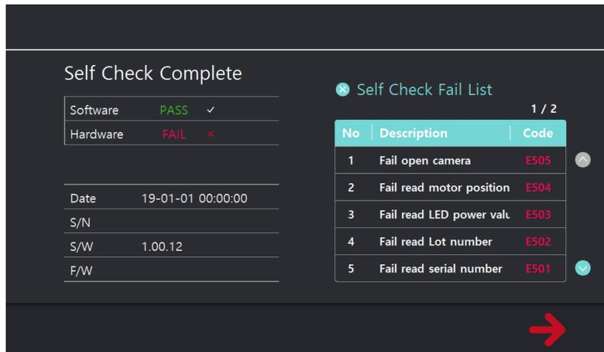
[Fig. 5] Self Check - Fail screen
