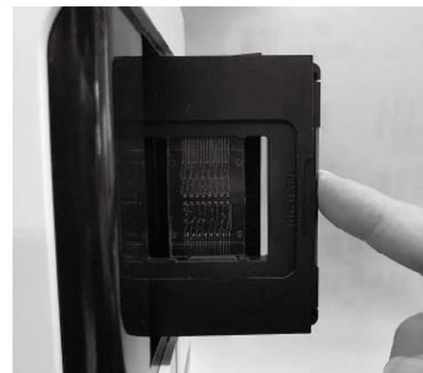
Gently push and insert it until a “click” sound is heard. (Caution – While the chip case is being completely inserted, do not forcibly push the chip case.)
